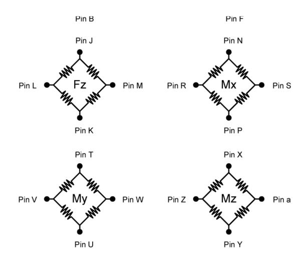
Bridges Fz; Mz = 700 ohms Bridges Fx; Fy; Mx; My; = 350 ohms **Connector Type:** Souriau 851-02E16-26P50-44
