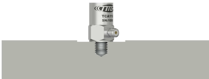
Figure 1. Stud Mounted Sensor
